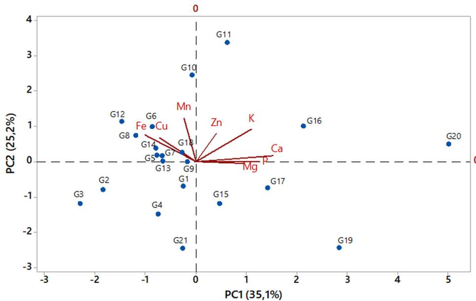
Figure 1. Scores and loadings biplot obtained from PCA data of mineral concentrations in geopolymer samples.
